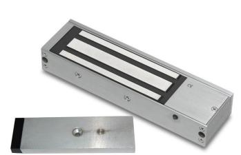
Standard single monitored magnetic lock, designed for indoor applications where 545kg holding force is required. Monitoring provides LED lock status indication and relay contacts for signalling. This model includes door status monitoring contacts to monitor the door position (open or closed).
