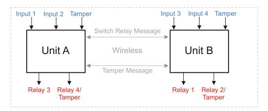
The Wireless Relay system has many applications where short range transmission of simple switches is required, for example, PA buttons, door contacts, remote sounders, lighting, door locking etc. The units are supplied in double gang plastic plates.
