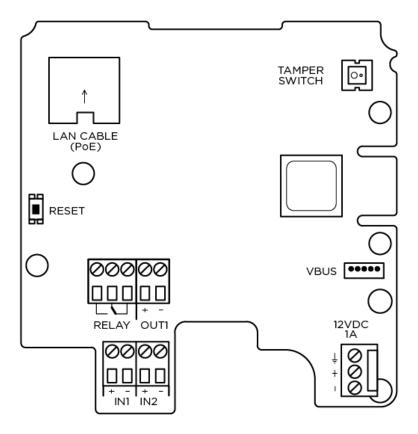
2N Access Unit Connectors, PCB Version 599v3
