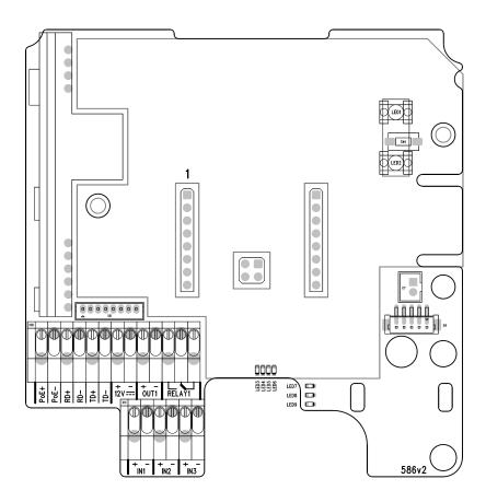
2N Access Unit Connectors, PCB Version 586v2
