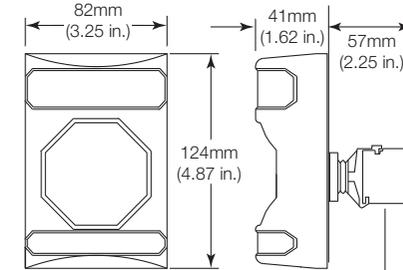
NOTE: MODELS REQUIRE KIT-71101B-\*COLOUR\* MODELS ONLY SUITABLE FOR EXTENDED DEPTH SURFACE MOUNTING DUE TO DIMENSIONS OF CONTACTS
