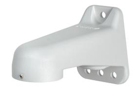
The WMVE-SR and WMVE-SW wall mounts can be installed directly to a wall or any vertical surface. Power and video wiring can be easily routed through the back of each mount or through the conduit access located on the bottom of the mount arm. The WMVE-SR/ WMVE-SW wall mounts can be adapted to pole mount applications using the PA101 pole mount adapter.
