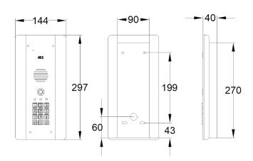
Stylish curved architectural model with Keypad. BS316 marine grade, brushed stainless steel construction with gloss acrylic faceplate. Kit includes 1 stylus **AUDIO** handset, 1 speech panel and 2 power supplies.
