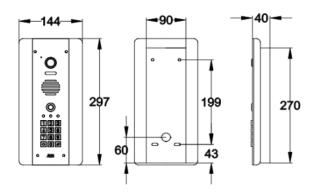
Stylish curved architectural model with keypad. BS316 marine grade, brushed stainless steel construction with gloss acrylic faceplate. Kit includes 1 stylus monitor, 1 speech panel and 2 power supplies.
