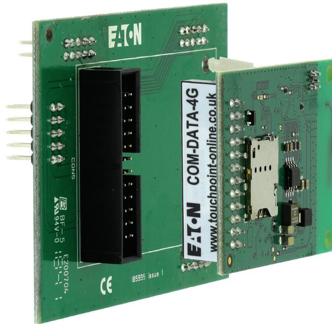
The COM-DATA-4G is a plug-on module that allows a control unit to access the Eaton SecureConnect™ service over the internet using LTE and GSM (4G and 2G) mobile phone networks.
