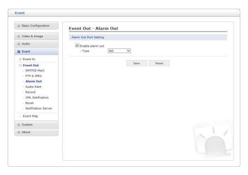
When the network camera detects an event, it can control external equipment connected to its alarm output port.
