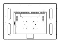
4) Mount the PVM27CAM/PVM32CAM to bracketry suitable for the application using either the VESA100 x 100 or VESA200 x 100 on the rear
