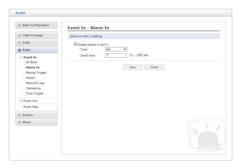
This camera provides 1 Alarm In port and user can set the port. The Port can be given as Normally Open or Normally Close state, and its Normal state can be configured. In order to use the alarm port, check the "Enable alarm port 1" first.
