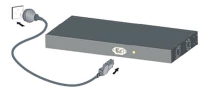
The AC power connection LED will show when power is applied.
