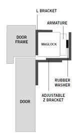
This adjustable Z & L bracket set provides a simple fixing method for slim fire rated maglocks on inward opening doors. The Z bracket is adjustable to cater for recessed doors.
