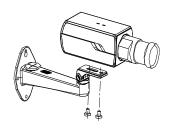
$\ensuremath{\textcircled{4}}$  Wiring, adjust the screws to adjust the camera's direction.
