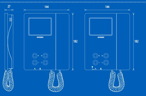
The 6200 series surface mount videophone with a 3.5" Hi-Res full colour active matrix LCD screen is designed primarily for low high-rise private developments and individual houses where an attractive low cost functional videophone is desirable.
