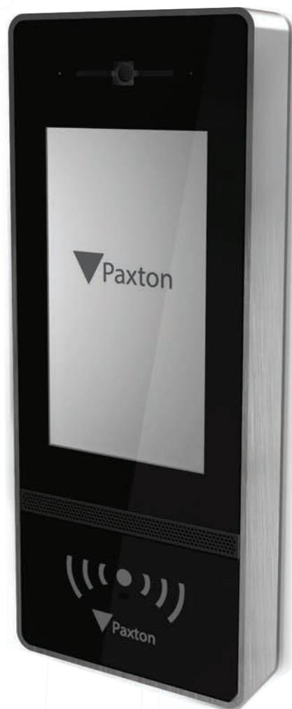
The Net2 Entry panel is a robust door entry panel incorporating both door entry and access control functions. It is powered using power over Ethernet (PoE) and communicates with the other elements of the system using IPv6, providing 'plug and play' installation. Each panel is associated with a Net2 Entry control unit which is the interface to the door hardware.
