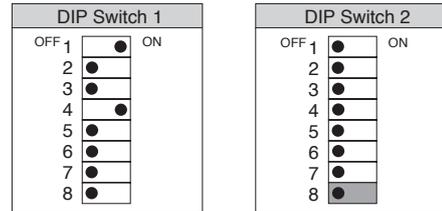
\*Keep the setting OFF in 8 of mode selector 2 for operation.
