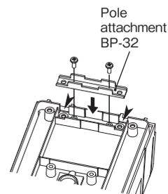
When using the pole attachment BP-32 (sold separately), break the knockout on the rear side of the sensor unit, and attach it.
