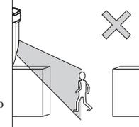
! After installation, make sure to adjust the detection area and perform sufficient operation check.
