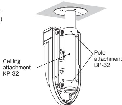
When mounting on the ceiling or under eaves, use the ceiling attachment (sold separately).
