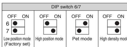
Low position mode : Select when the installation height is 6.6' to 9'(2.0 to 2.7m.)
