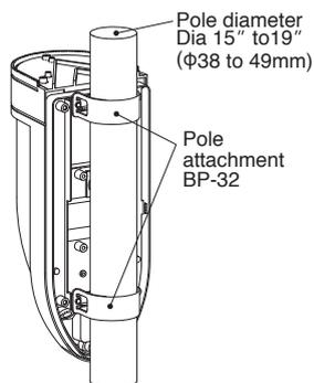
When mounting the unit on a vertical pole, use the pole attachment (sold separately). The unit can be mounted on poles of Dia 15" to 19" (φ 38 to φ 49mm) and Dia 15.7" to 55" (φ 40 to φ 140mm).
