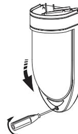
\*When installing outdoors, mount the anti bird spike above the cover unit. Turn the anti bird spike and tighten it.
