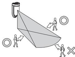
Set the area within the rated detection distance range according to the instruction manual. If you use the unit outside the specified range, an appropriate area will not have been configured, and the unit may operate unsteadily, and/or detection may fail.
