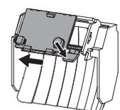
Unlatch the alignment lever and return to its original position
