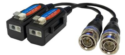
The Vista VBALUN-4KPOC video baluns are passive (non-amplified) devices allowing transmission of real-time CCTV analogue HD video formats including CVBS, TVI, CVI and AHD up to 4K resolutions over Unshielded Twisted Pair (UTP) cabling.
