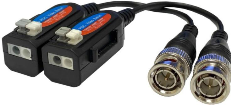
The Vista VBALUN-4KPOC video baluns are passive (non-amplified) devices allowing transmission of real-time CCTV analogue HD video formats including CVBS, TVI, CVI and AHD up to 4K resolutions over Unshielded Twisted Pair (UTP) cabling.
