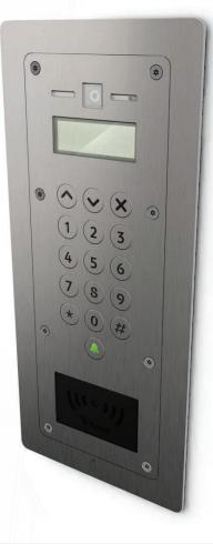
The Entry panel is a robust door entry panel incorporating both door entry and access control functions. It is powered using power over Ethernet (PoE) and communicates with the other elements of the system using IPv6, providing 'plug and play' installation. Each panel is associated with a Entry control unit which is the interface to the door hardware.
