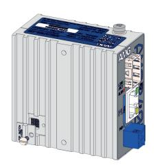
Remove DIP switch cover to access 4 DIP switches.
