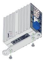
Attach the supplied wall bracket using 2x M3×4mm screws included in the box. Multiple mounting options are available:
