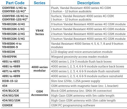
\*Multiple button panels (up to 24 buttons) can be achieved using a combination of the VR4K series button modules with the appropriate **VR4KGSM-n/4G** entry panel and 4000 series flush or surface back boxes.
