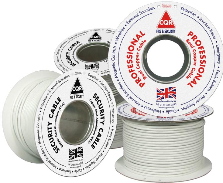
A new range from CQR which has been designed, tested and manufactured in the UK for domestic applications and is suitable for shorter runs. This cable is based on cores made from 7 strands of 0.2mm Copper Clad Aluminium Magnesium (CCAM) and is sheathed in Type 1 PVC.
