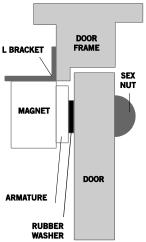
This architectural L-bracket has a curved cover that gives an aesthetically pleasing appearance. Use on outward opening doors to fix the magnet to the door frame. Multiple fixing points enable the magnet to be fixed in the optimum position.
