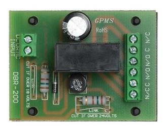
This relay board provides a very convenient method of switching two independent circuits via a controlled on/off input voltage. The relay provides double-pole-double-throw dry contacts, and is commonly known as a 'very handy little relay', or VHLR.
