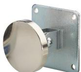
This wall mounted door retainer is ideal for holding open doors in corridors that need to be closed on activation of a fire alarm (a spring door closer is required in addition). It has a push button that enables manual release when required.
