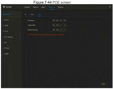
Step 2 The NVR will deploy IP addresses to the cameras which connect POE immediately.
