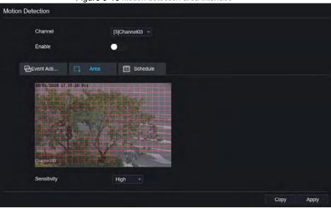
Figure 9-18 Motion detection area interface
