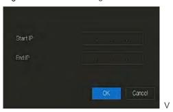
Step 5 Enter value manually for start IP address, end IP address.
