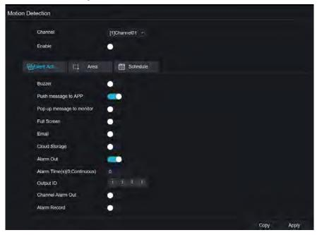
Figure 9-17 Motion detection interface
