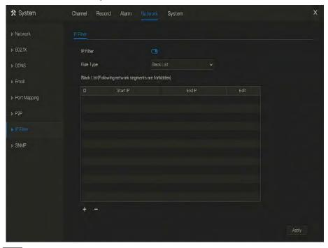
Figure 7-52 IP Filter setting screen
