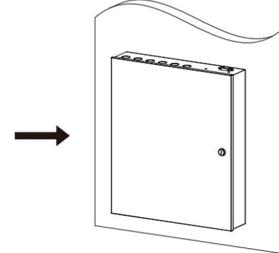
3 Close the chassis cover to complete the installation.
