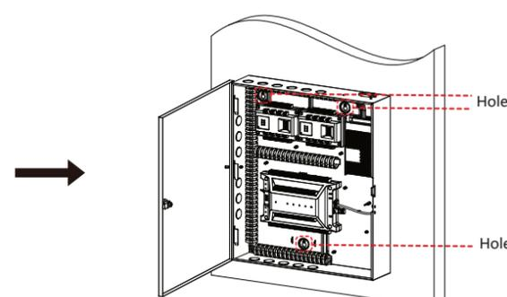
2 Open the chassis cover and press the holes on the chassis body with the screws reserved on the wall. Then attach the chassis from top to bottom onto the screws.
