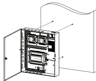
1 Fix 3 SC-KA4X45 screws to the wall, and 3 to 5 mm thread should be reserved on the top of the screw (to facilitate subsequent hanging of the chassis).
