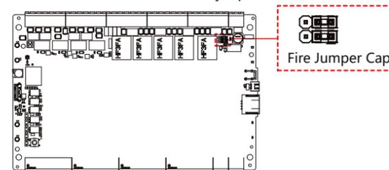
The position of the fire jumper cap position and the related NO/NC status are as follows:
