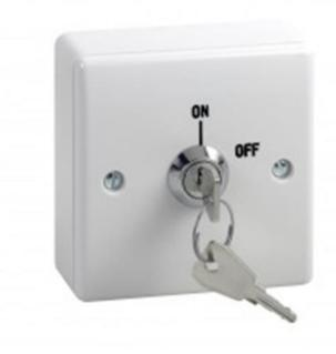
Double pole, maintained key switch, ideal for overriding door access control systems. The key is removable in either the 'on' or the 'off' position.
