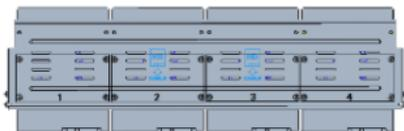
4. Put the mounting plate back in place. Connect power and data cables as shown below. Repeat the steps to connect all the disks.
