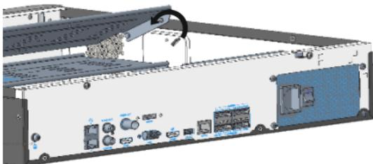
3. Secure the disks on the mounting plate. Fix the screws according to the figure below and avoid damaging the disk in the process.
