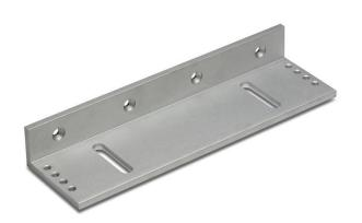
This L-bracket is designed to enable a 'standard' maglock to be fixed to the door-frame of an outward opening door. Multiple fixing points enable the magnet to be fixed in the optimum position.
