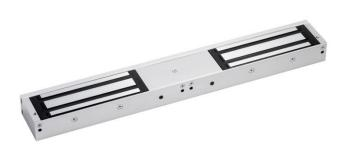
Standard monitored double magnetic lock, designed for indoor applications where 545kg holding force is required. Monitoring provides LED lock status indication and relay contacts for signalling.
