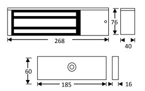
Standard single monitored magnetic lock, designed for indoor applications where 545kg holding force is required. Monitoring provides LED lock status indication and relay contacts for signalling.
