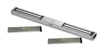
Double Slim unmonitored magnetic lock with door status. Compact design, making it ideal for most indoor applications where 250kg holding force is sufficient (each side).
