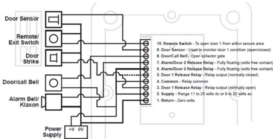
**Note:** When making connection to the door strike, select 'relay normally open' or 'relay normally closed' to suit the intended application and locking mechanism.
