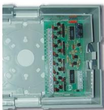
Two interface cards are available to enable Multiguard annunciators to drive external equipment.
