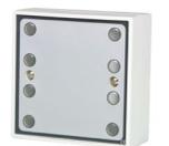
The **EXITGUARD 200 Series** uses a nine-digit keypad for both control and programming. The tone of the high power integral alarm can be selected to distinguish it from other alarms. The alarm can be silenced and reset using a four-digit code or the EXITGUARD can re-arm automatically after a pre-set delay once the door has been closed. Separate Door Open Too Long (DOTL) delays can be set for Code Reset and Auto Reset modes. There is also a Bleep In Off option and Chime facility.
