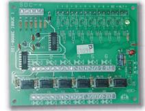
**MG311000 Nurse Call annunciators** - The principle of operation is similar to the Multiguard general purpose annunciators. There is a SILENCE button F1 but no reset button or isolate facilities are fitted. Integral power supplies are NOT usually fitted to these versions as extra power is needed for call points and overdoor lights etc...
