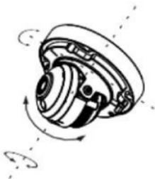
7. Re-fit the domes bubble to the camera using the reverse of the procedure you followed in step 2 – remembering to refit the trim ring if one was included.
