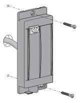
If the reader is fitted with screw terminals, position the reader against the mounting surface, ensure that the reader is level and mark out the position of the fixing holes. Drill and prepare the fixing holes. Feed the connecting cable through the cable hole and terminate the conductors according to the wiring details overleaf.
