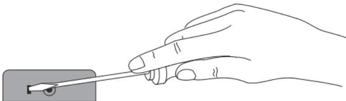
Insert the tip of a terminal screwdriver into the small slot in the base of the cover. Press lightly to release the securing catch while you separate the cover from the reader at the base.
