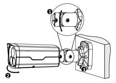
3. Once correct position and field of view is achieved, tighten both lock screws and large locking collar (3).
