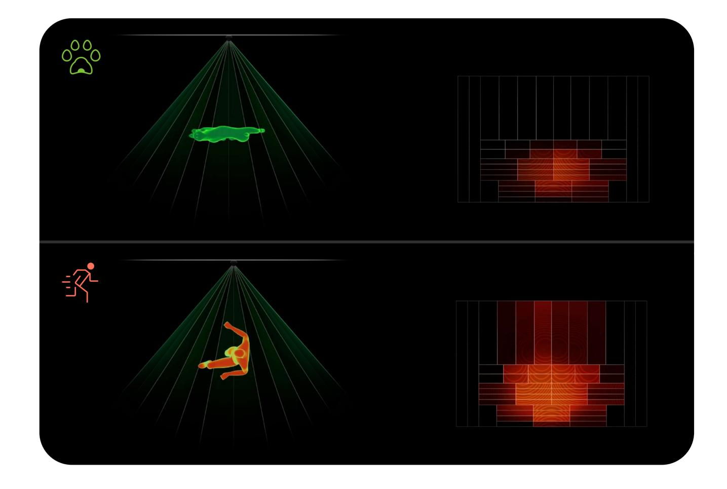
analyses the thermal diagram from the PIR sensor: the intensity of IR radiation, the size of the thermal spots, the speed of movement and other parameters.
