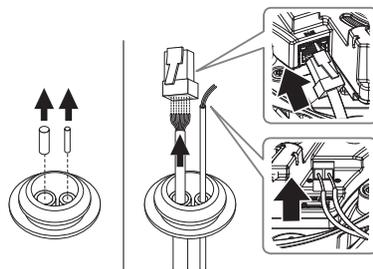
5. Insert the cable bushing of the audio/alarm cables into the camera body.
