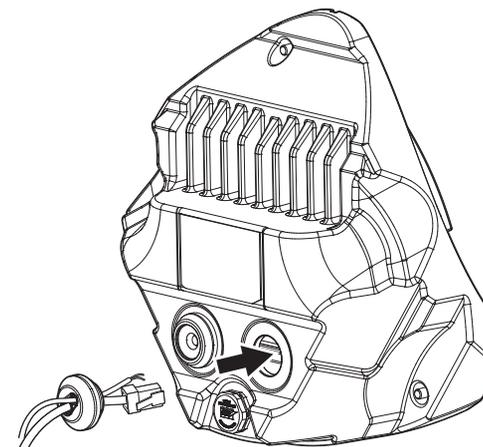
[Installing audio/alarm cables]
