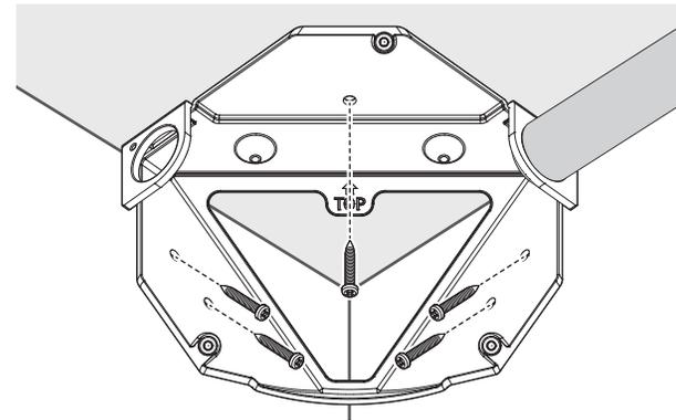
2-3. Pull out network cable through the pipe.
