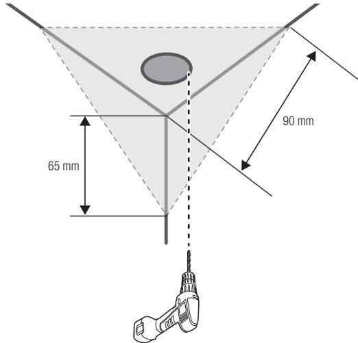
1-2. Fix the mount bracket by using the appropriate screws.
