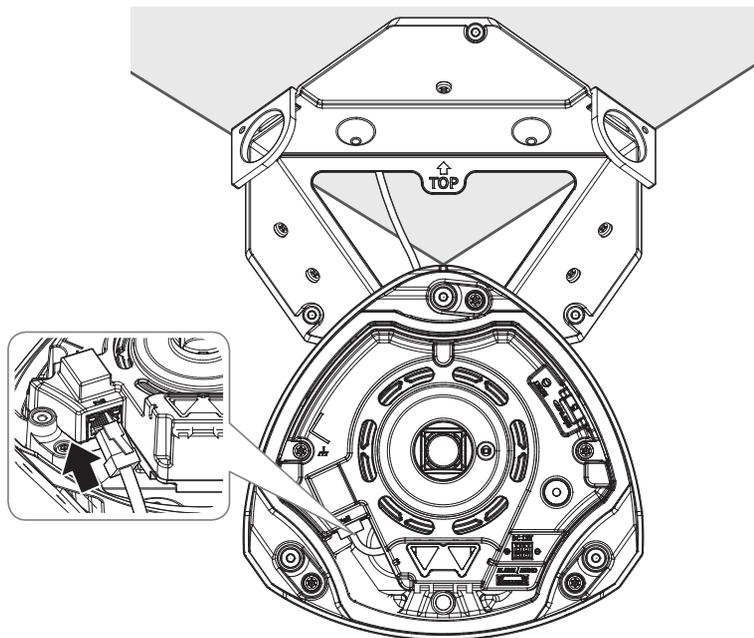
3-4. Mount the cable bushing to the camera body.
