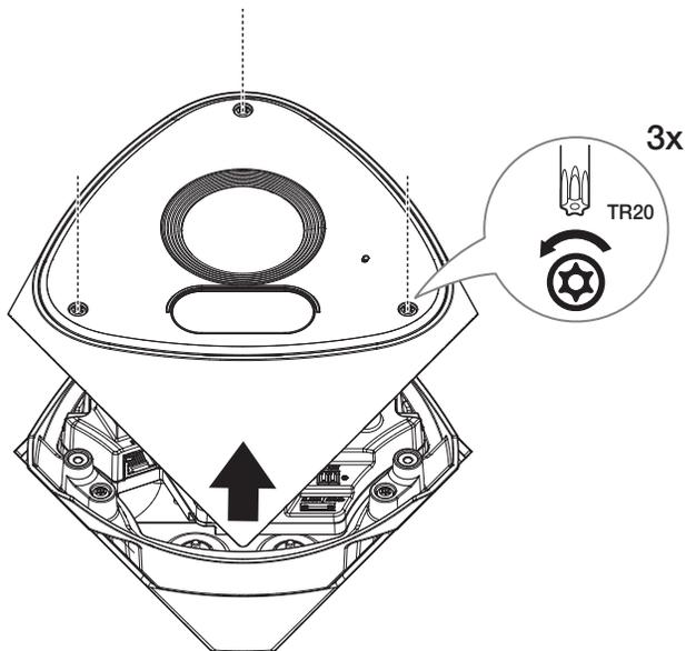
2. Remove the camera body by turning its fastening screw counterclockwise.
