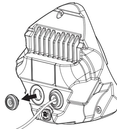
[Installing network/power cables]
