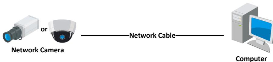
Figure 2-1 Connecting Directly
