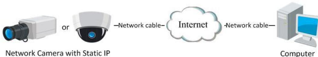
Figure 10-2 Accessing the Camera with Static IP Directly
