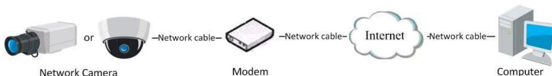
Figure 10-3 Accessing the Camera with Dynamic IP
