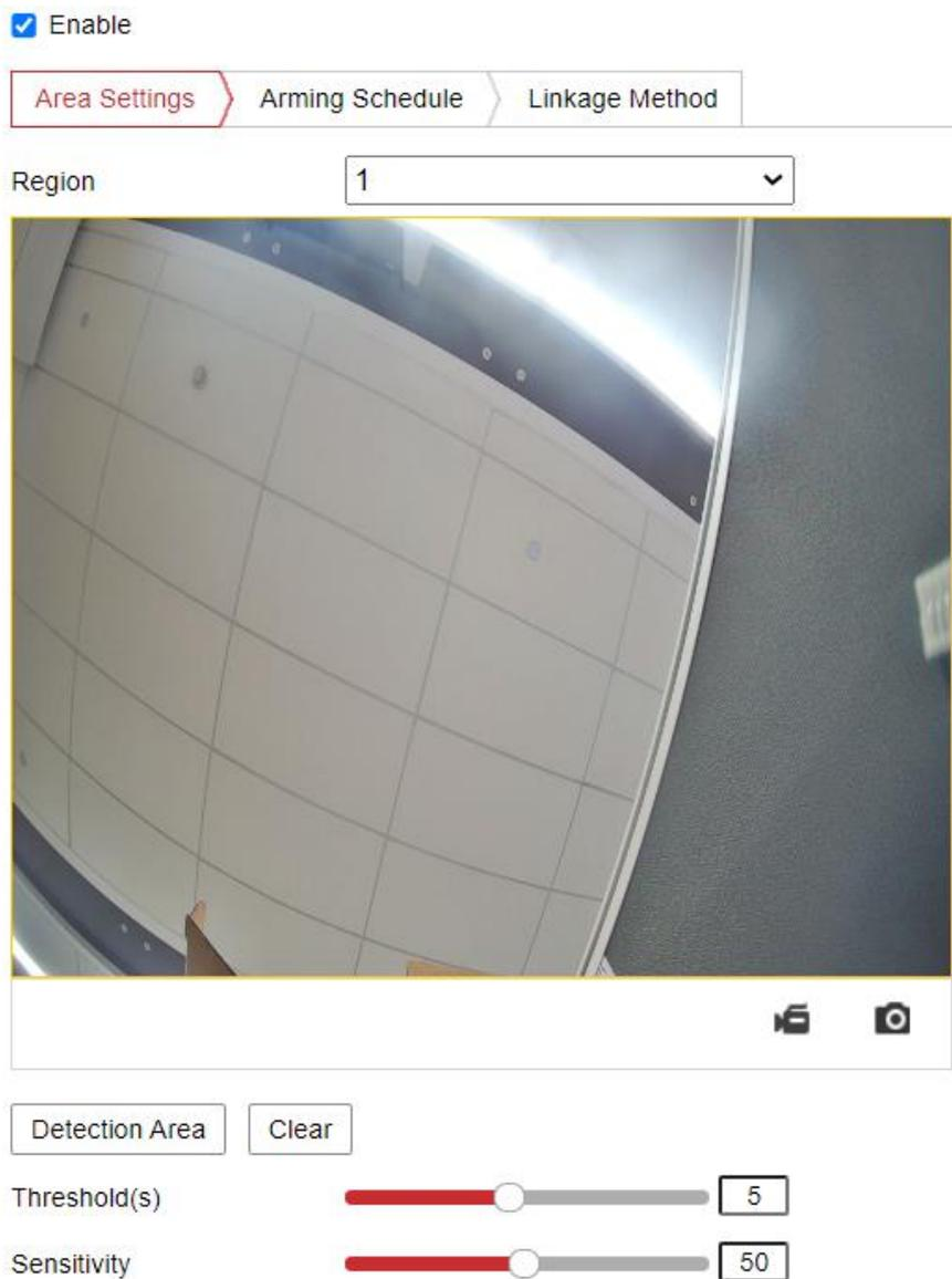
Figure 8-17 Loitering Detection
