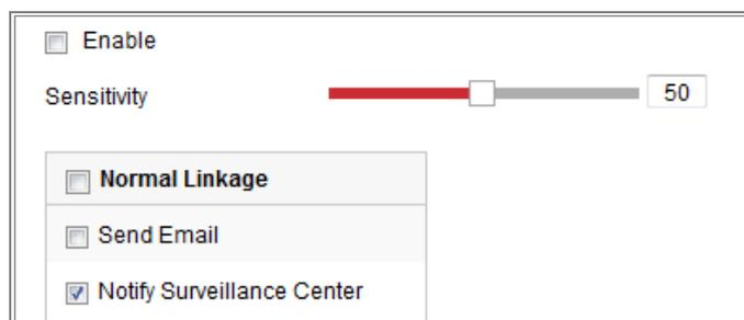
Figure 8-8 Defocus Detection
