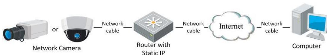
Figure 10-1 Accessing the Camera through Router with Static IP
