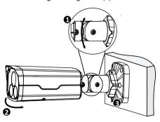
3. Once correct position and field of view is achieved, tighten both lock screws and large locking collar (3).
