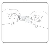
Remove the tag's protection layer. Avoid touching the adhesive side as much as possible.
