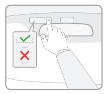
Ensure that the tag is positioned horizontally and in line of sight of the reader.
