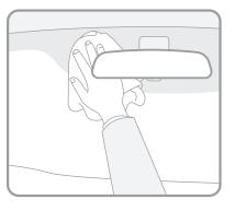
Clean the inside surface of the windscreen. Make sure the windscreen is completely oil and dirt free.
