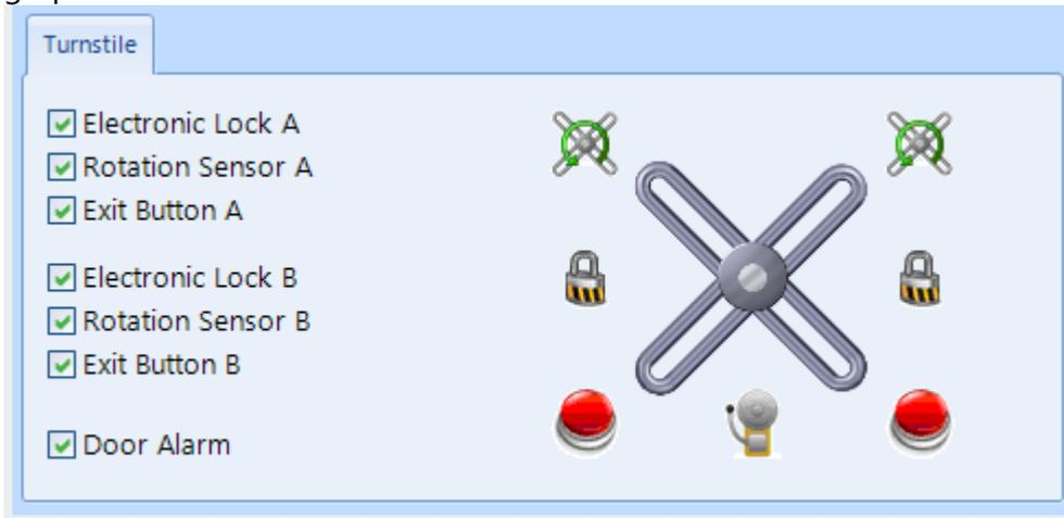
The components required for the turnstile to operate are:
