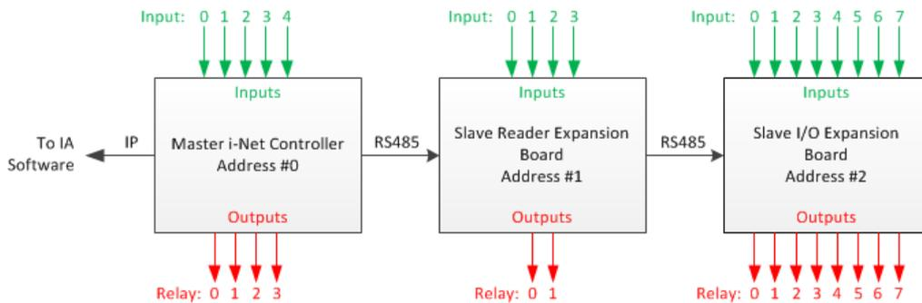
The channel comprises of an i-Net controller connected to the Identity Access software via IP. This is called the Master i-Net.
