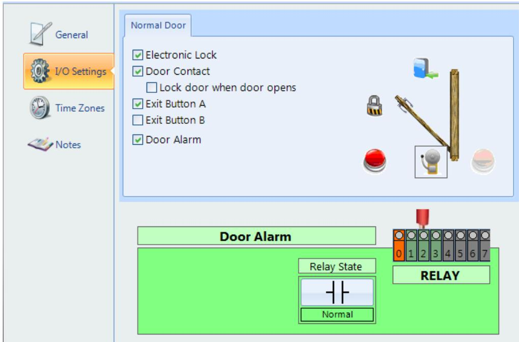
If **Relay State** is **Normal**, the relay will energise to activate the sounder. Conversely, **Inverted** will de-energise the relay to activate the sounder.
