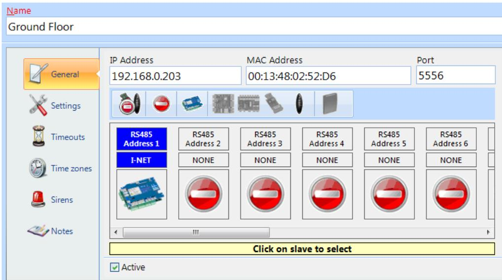
This information will then be used during the programming to define which inputs, outputs etc. are available for use. **NOTE: Slave i-Nets and expanders cannot be combined on a single RS485 bus. Selecting a Slave i-Net greys out other expanders (and visa versa) reducing the possibility of configuration errors.**
