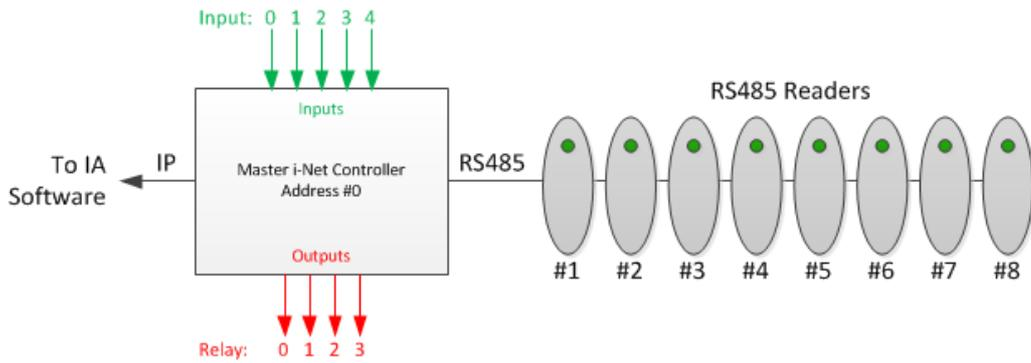
The channel comprises of an i-Net controller connected to the Identity Access software via IP. This is called the Master i-Net.
