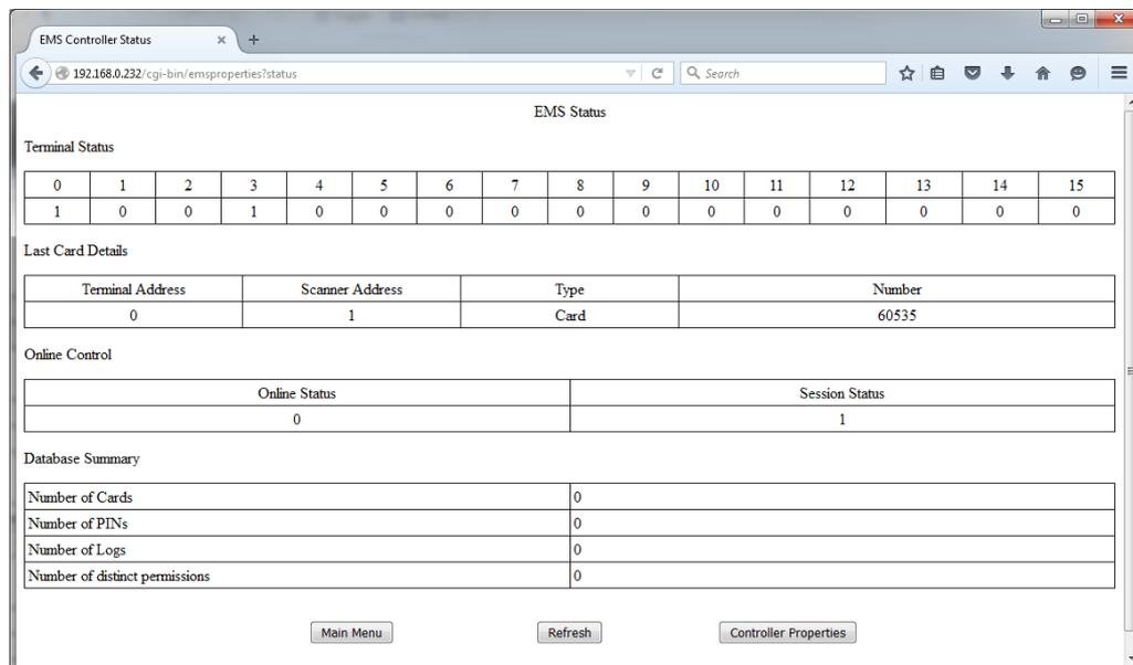
**Terminal Status** displays the devices connected to the i-Net's RS485 bus. In this example, we have device address 0 (the Master i-Net itself), and a device with address 3.
