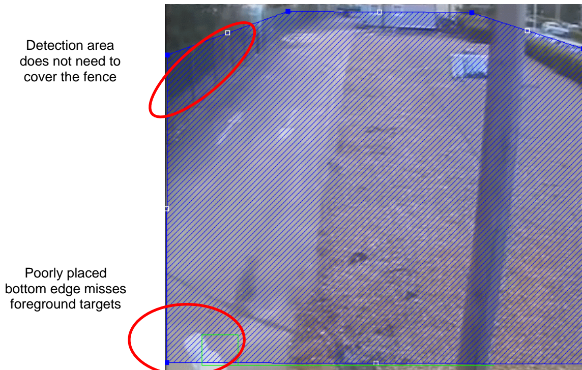
Figure 4: Poor Detection Area Placement
