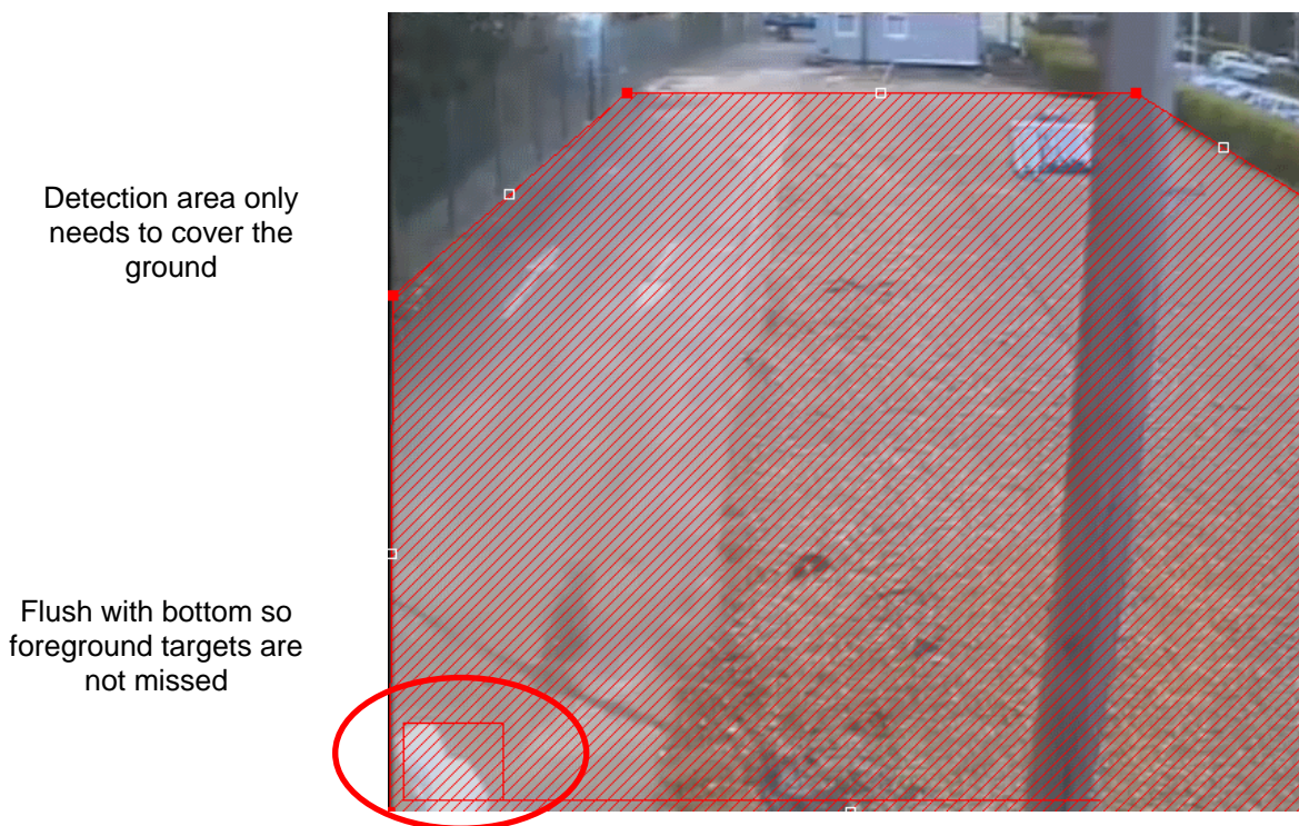
Figure 5: Good Detection Area Placement
