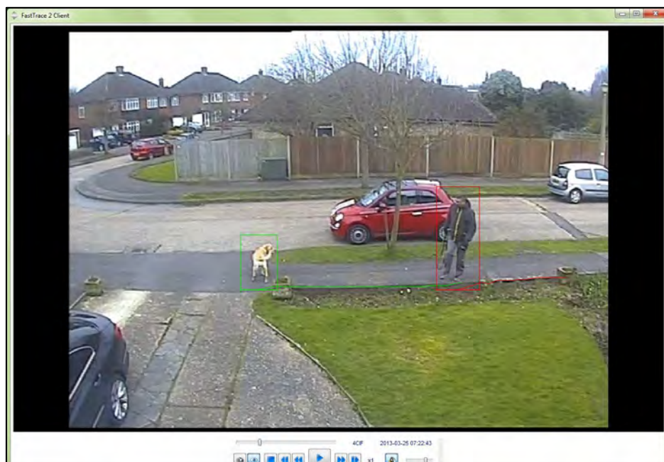
Figure 16: Example Showing Man Detected while Dog is Ignored
