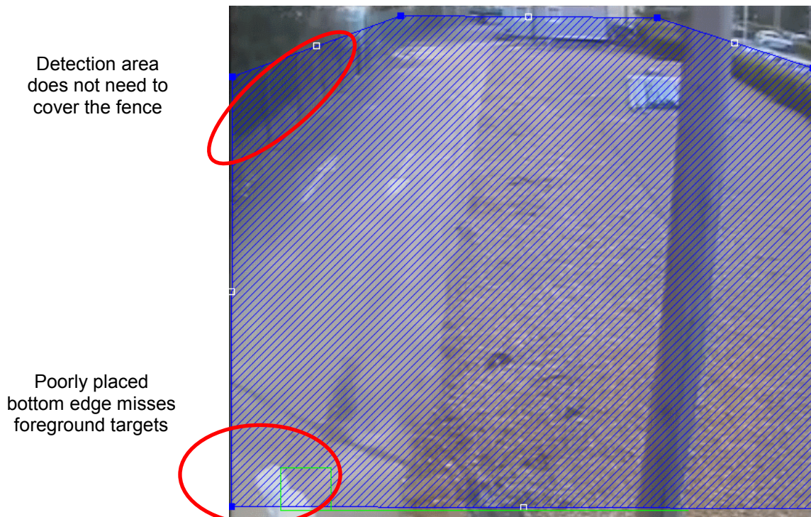
Figure 5: Poor Detection Area Placement
