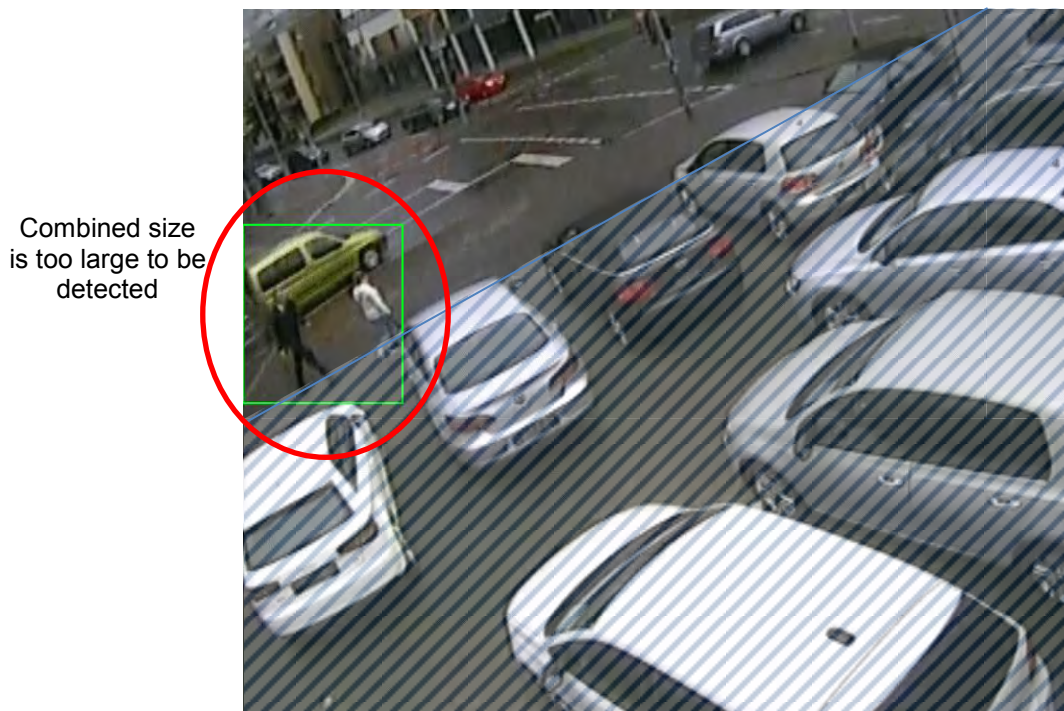
Figure 23: Traffic Interfering with Pedestrian Detection
