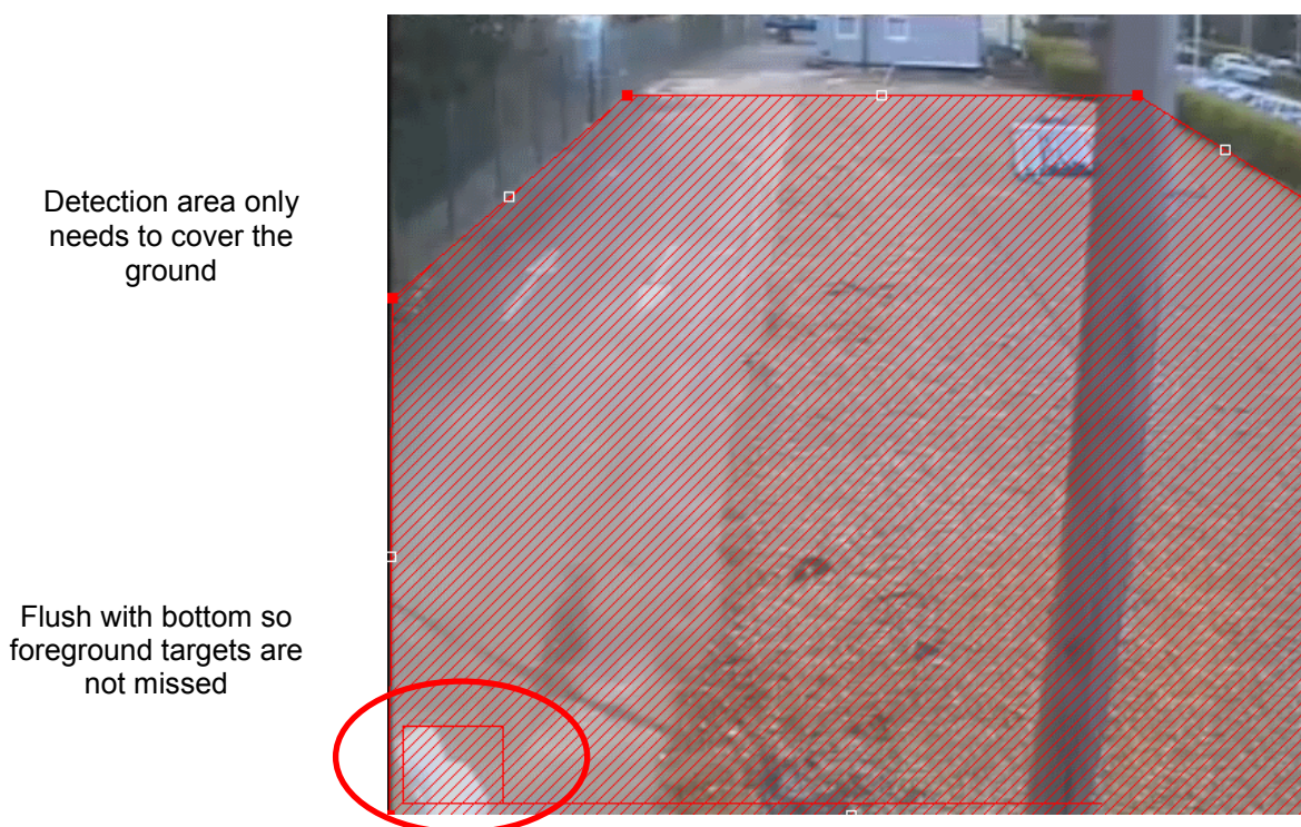
Figure 6: Good Detection Area Placement
