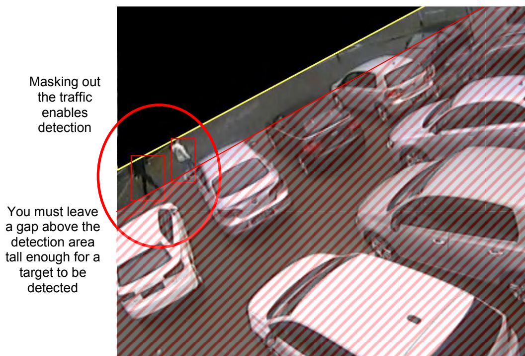
Figure 24: Effective Masking of Traffic
