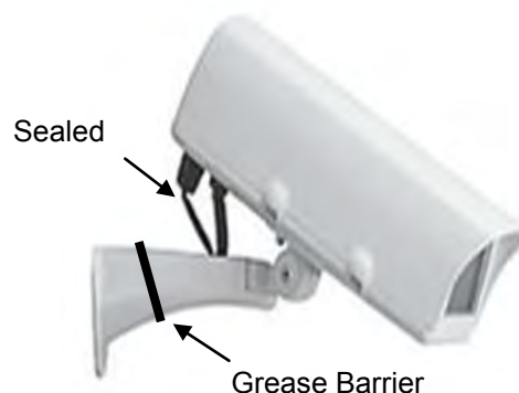
Figure 28: Possible Solution using a Grease Barrier
