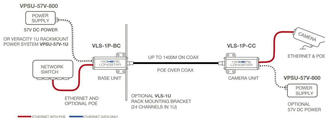
POE Models of HIGHWIRE Longstar enable both network data and power to be carried over extended lengths of new or existing coaxial cable.
