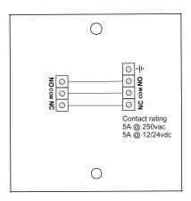
Terminals will accept cable sizes up to 2.5mm², however 1mm<sup>2</sup> is recommended
