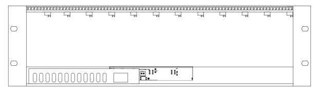
The **AMG2015** is a subrack for a standard 19" rack. It is designed to house rack-mount AMG3000-5000 series video transmission equipment.
