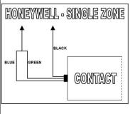
Ensure that unused/trimmed wires are insulated. Shorting of unused wires will affect operation.
