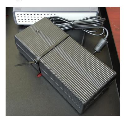
5. Connect power supply barrel connector to power jack at back of switch
