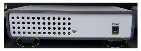
3. Secure switch using screw and washer on left and right side of front of switch
